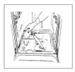
The salt container must be filled when the "low salt" indicator light (located on the control panel) comes on.
